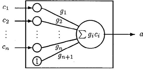
Figure 4: An instance of the linear controller.  $g_i$  denotes a feedback gain which is characterized by  $w_i$  according to  $g_i = w_i + N(0, \sigma^2)$ . The controller learns  $w_i$  to achieve good control.
