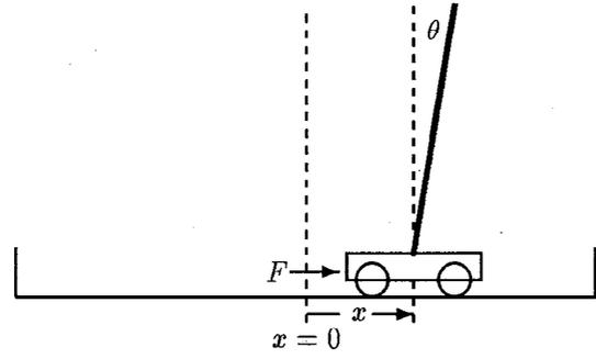
Figure 5: A simulation model of the cart-pole task.
