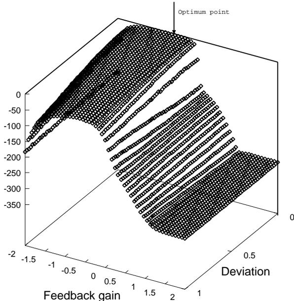
Figure 9: Value function over the parameter space in the LQR problem, where  $\gamma = 0.9$ . It is fairly flat around the optimum:  $\mu = -0.5884$ ,  $\sigma = 0$ .
