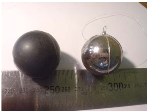
Fig.4 The targets of the measurement: A rubber ball and a metal ball.
