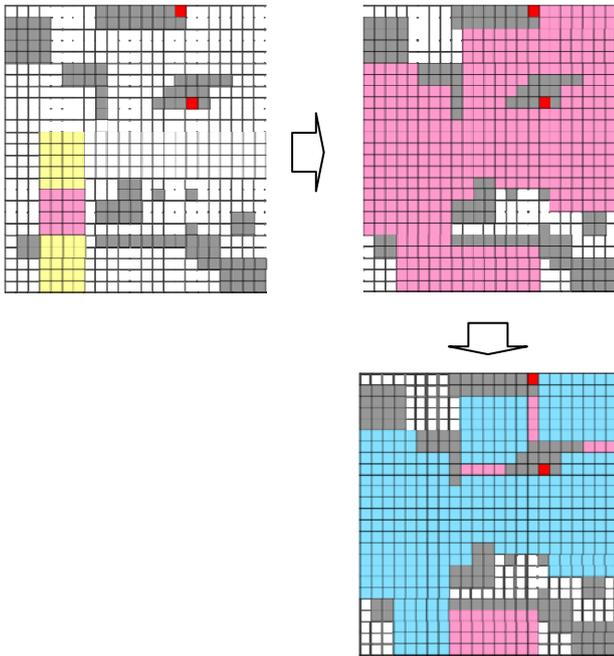
Figure 5: Recursive fill algorithm to find accessible space
