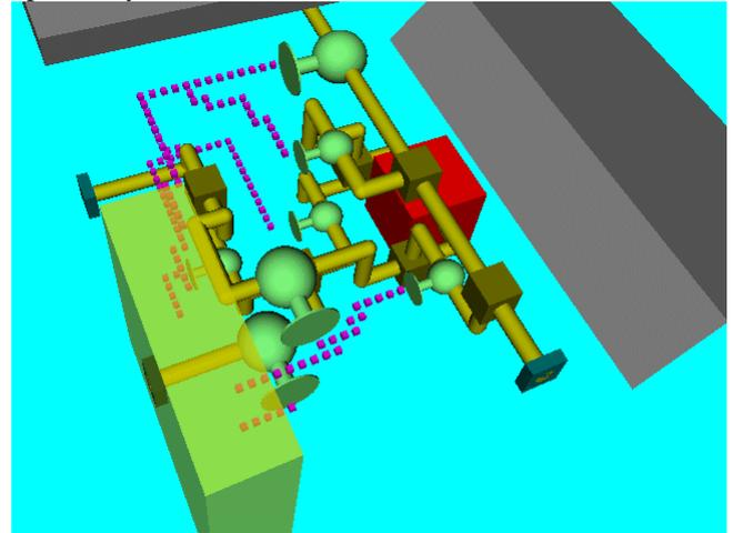
Figure 10: A solution in the problem of 7-valves
