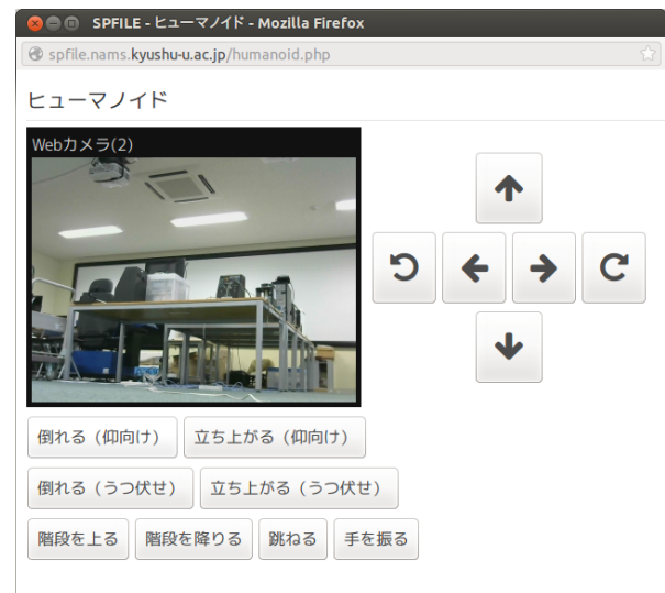
Fig. 3 A web page for the robot control
